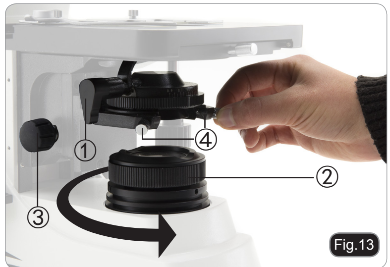
CENTERING THE CONDENSER
